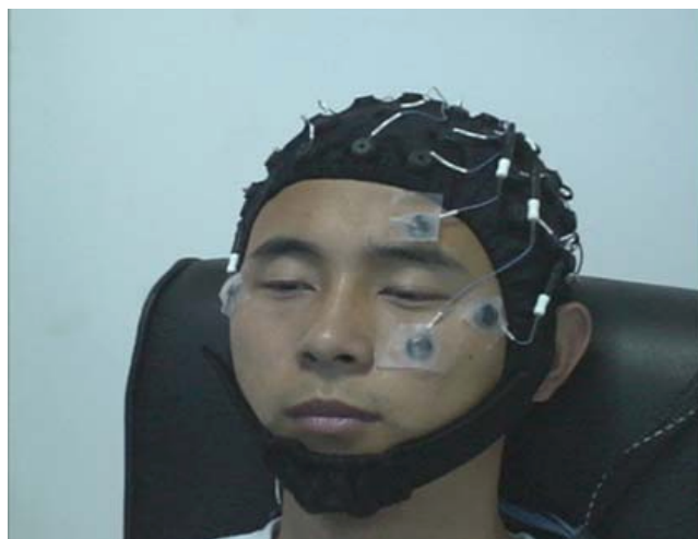
Fig. 4. The subject wears a special hat with 64 electrodes connected to the amplifier of the NeuroScan system. The four electrodes attached to the face of the subject are used to record EOG.
