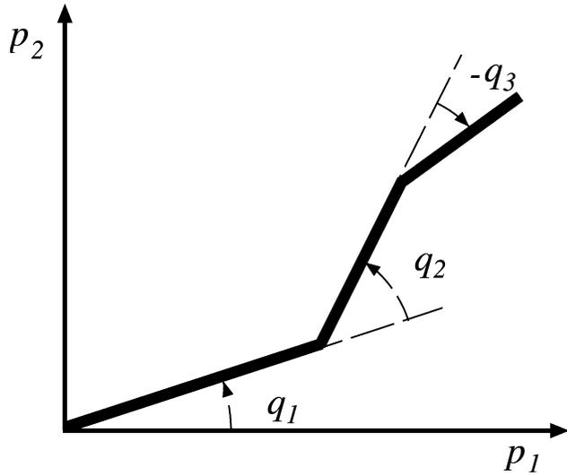
Fig. 4. A three-joint planar manipulator.
