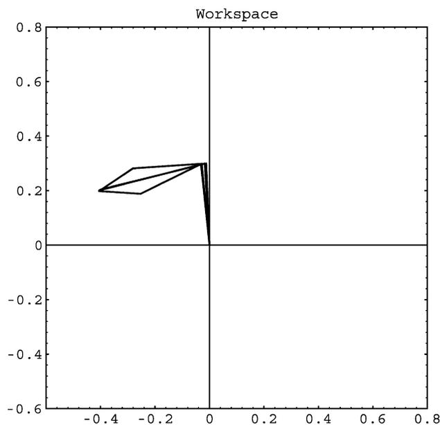
Fig. 5. Four different inverse kinematic solutions obtained by solving the SP problem defined by Eq. (34). Note that two of solutions are quite near and overlapped in the figure.
