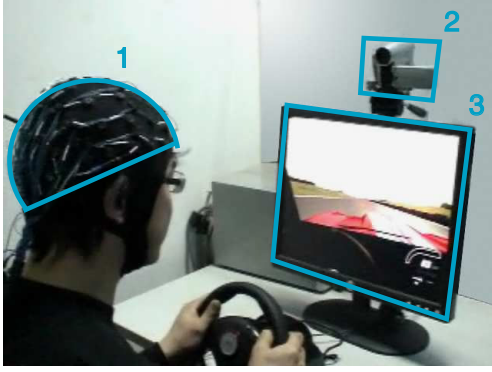
Fig. 1. Driving simulation environment. Here EEG signals are captured from scalp by the electrode cap (1), the subject's face expression is recorded by a DV (2), and driving scenes are displayed on the LCD screen (3).
