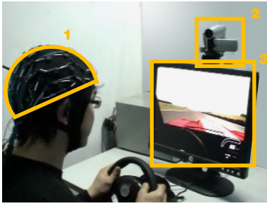
Fig. 1. Driving simulation environment. Here EEG signals are captured from scalp by the electrode cap (1), the subject's face expression is recorded by a DV (2), and driving scenes are displayed on the LCD screen (3).
