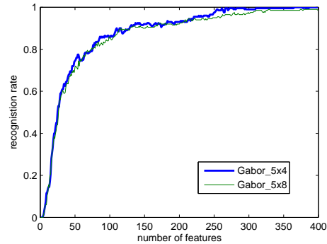
Fig. 3. Face recognition performance of the PCA method with two different sets of Gabor filters: \text{Gabor}_5 \times 4 and \text{Gabor}_5 \times 8 .
