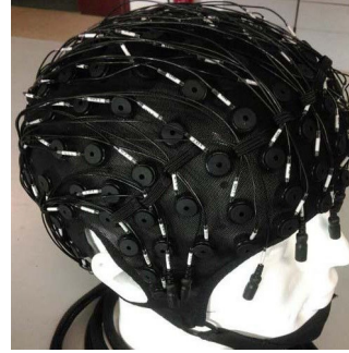
(c) Wet electrodes EEG cap
