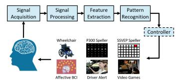
Fig. 1. Flowchart of a closed-loop EEG-based BCI system.
