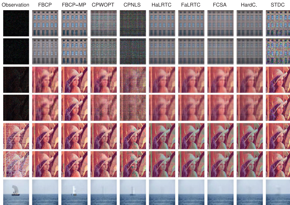
Fig. 6. Visual effects of image inpainting. Seven examples shown from top to bottom are (1) facade image with 95 percent missing; (2) facade image with 95 percent missing and an additive noise; (3) Lena image with 90 percent missing; (4) Lena image with 90 percent missing and an additive noise; (5) Lena image with superimposed text; (6) scribbled Lena image; (7) an image of ocean with an object.
