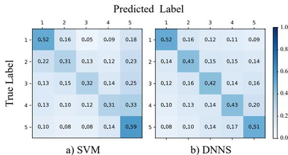
Fig. 3. Confusion matrix of the two classifiers for the five decision confidence levels with the DE feature. The rows represent the target class, and the columns represent the predicted class.
