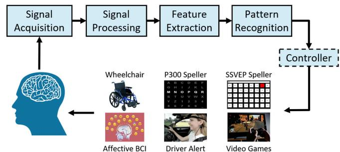
Fig. 1. Flowchart of a closed-loop EEG-based BCI system.
