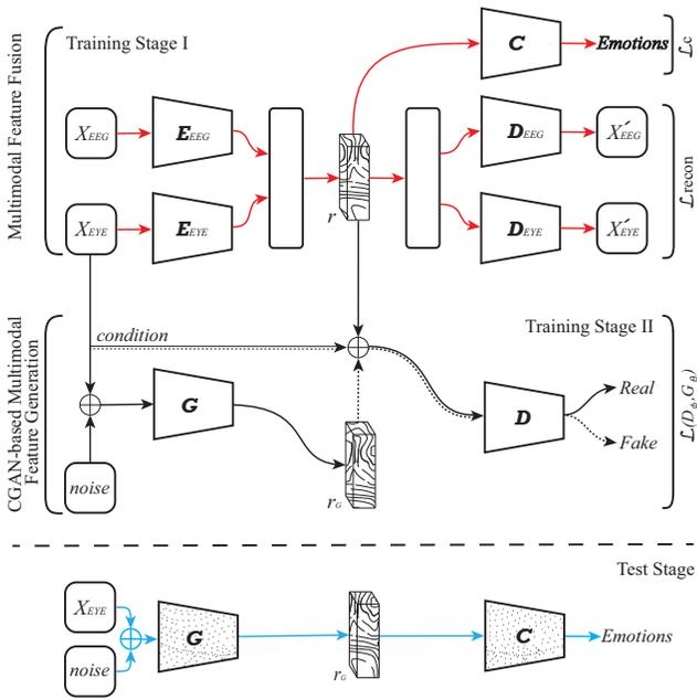
**Figure 1: The framework of our system. The training stage can be divided into two parts as multimodal feature extraction and multimodal feature generation. In the test phase, only eye movement signals are needed. The shaded  $G$  and  $C$  indicate that they have been trained. Best viewed in color.**
