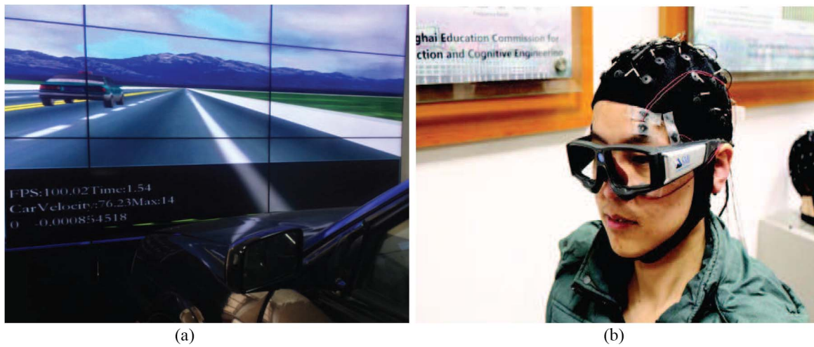
Fig. 1. Simulation experiment environment. (a) LCD screen. (b) SMI-ETGW and the electrode channels.
