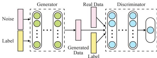
Fig. 2. Illustration of the proposed CWGAN, which consists of two parts: the generator generates realistic-like data and the discriminator distinguishes real and generated data. An auxiliary label information is concatenated to control the categories of the generated data.
