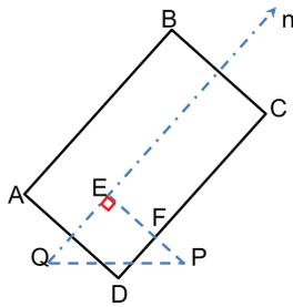
Fig. 11. Definition of cylindricity error.
