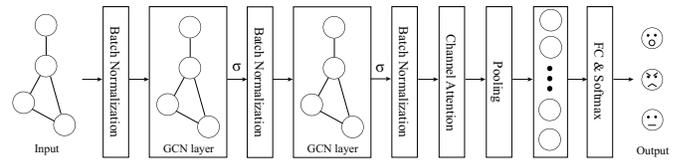
Fig. 2. The overall architecture of proposed GCNCA model.
